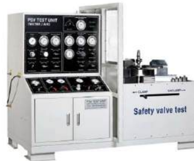
Mobile PSV & ValveTest Unit (On-site execution type) Test medium : N2 or Water Q'ty : x1set Total Price Value : 140,000.00 USD
