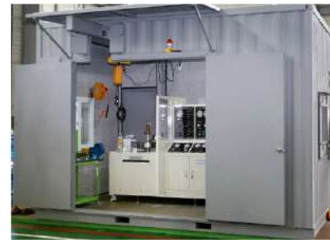
Mobile PSV & ValveTest Unit (On-site execution type) Test medium : N2 or Water Q'ty : x1set Total Price Value : 140,000.00 USD
